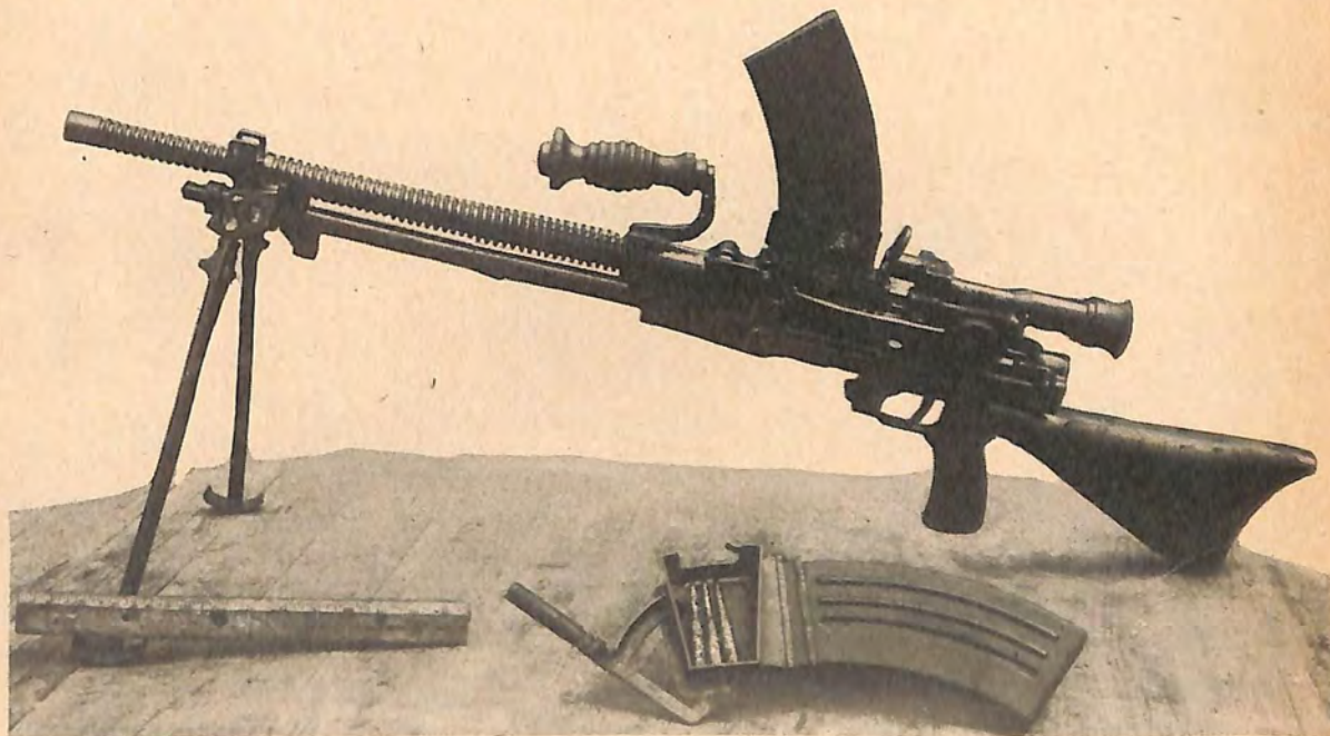
Figure 179. Model 96 (1936) 6.5-mm light machine gun (showing magazine, magazine filler and telescopic sight).
